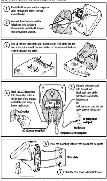
Note: To mount the phone directly on the wall, insert two 1 <sup>3</sup>/<sub>8</sub> inch, #10 screws (not supplied) into the wall using anchors suitable for the wall material. Place the screws 3 <sup>15</sup>/<sub>16</sub> inches apart, and allow <sup>1</sup>/<sub>8</sub> inch free space between the wall and screw heads.
